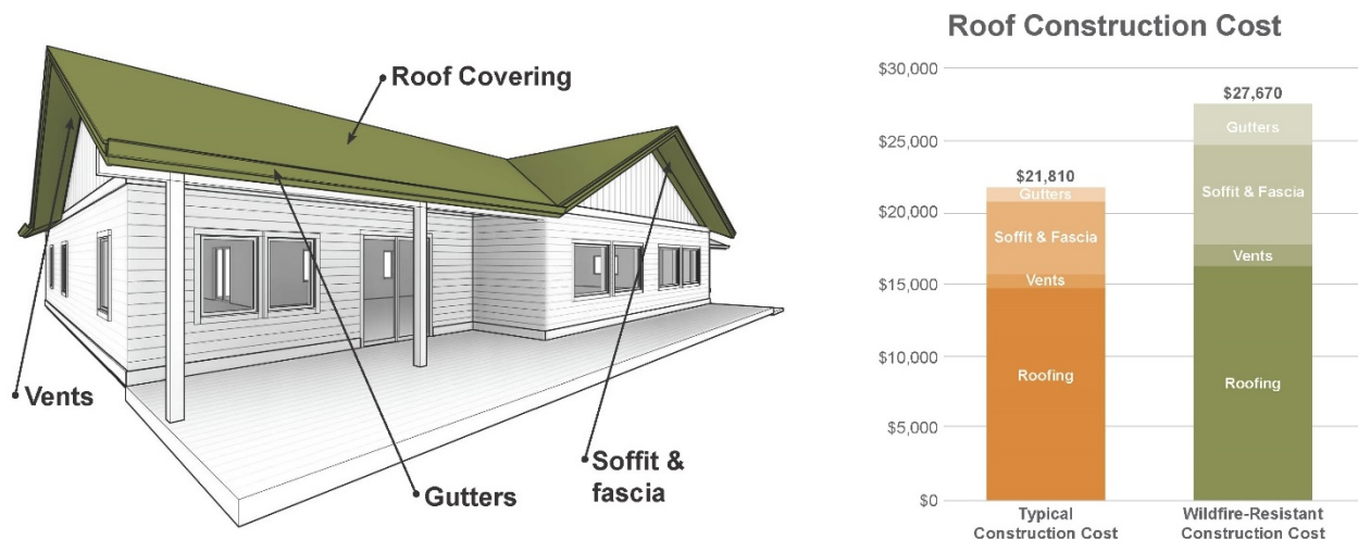
Figure 1.2. Roof subcomponents and new construction cost.
