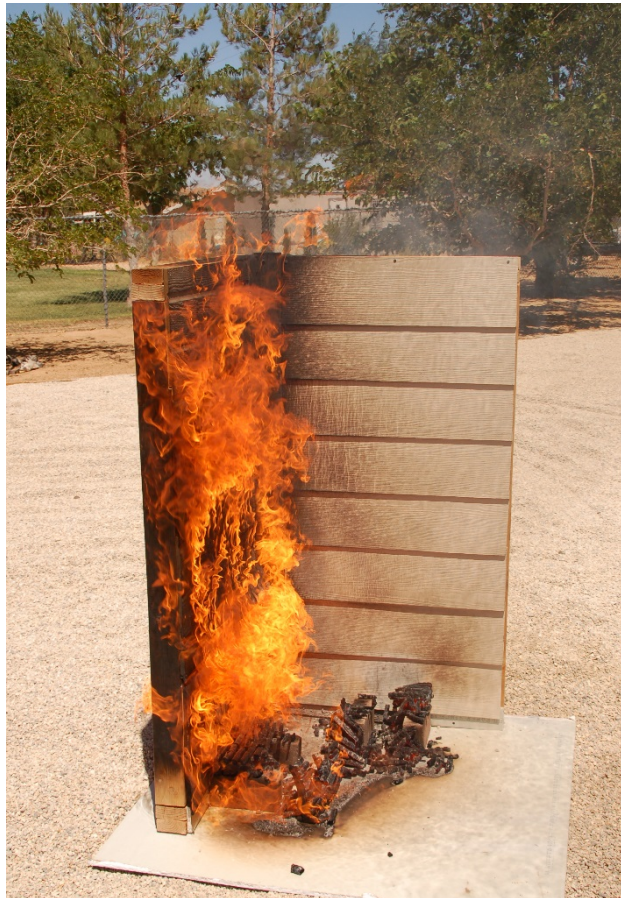
Figure 3.2. Vertical flame spread after exterior siding ignites can threaten other components on the wall, such as windows and the under-eave area. Photo: Stephen L. Quarles
